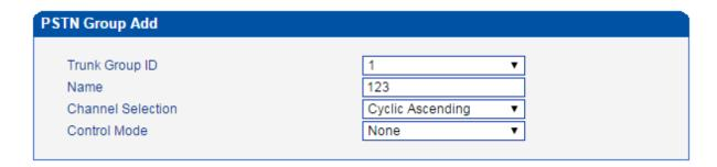
Step5. Enter into the **PSTN Group Management** interface to associate the PSTN profile and PSTN group to an E1/T1 port or multiple E1/T1 ports.
