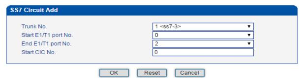
Note: If multiple E1/T1 ports are involved, it defaults that all the 32 channels of each E1/T1 port involved are used by the SS7 trunk.
